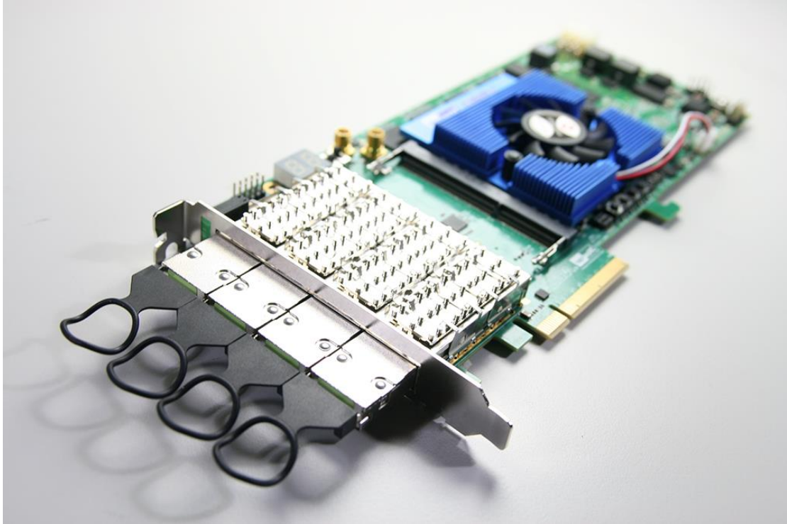
Figure 8-4 Four QSFP+ Loopback Fixtures Installed
